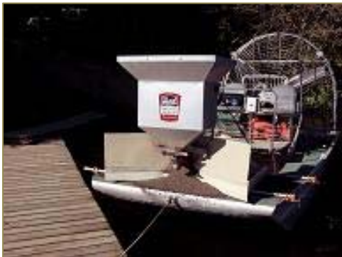
Figure 17. Herbicide application equipment
